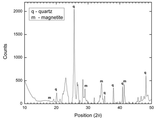
Figure 5. SR-XRD pattern for a black pigment specimen showing the presence of magnetite and quartz.
