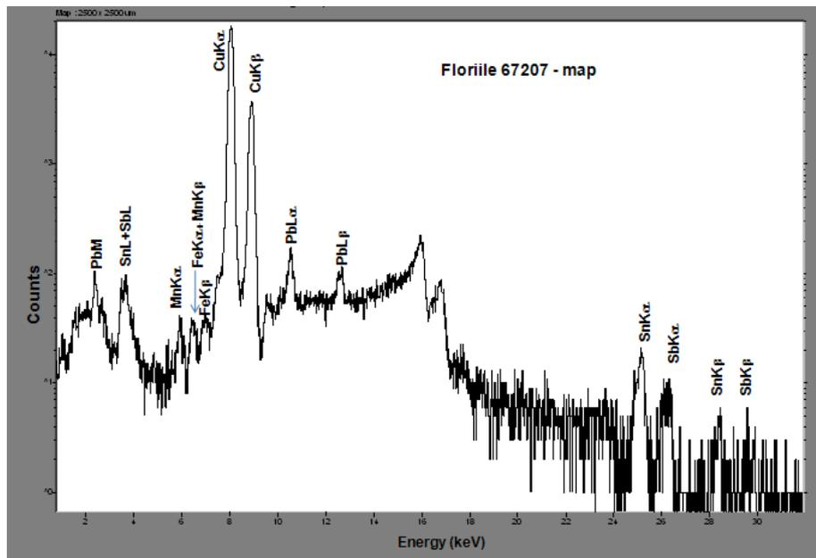
Fig. 5b – Floriile 67207 sample – micro-PIXE spectrum.
